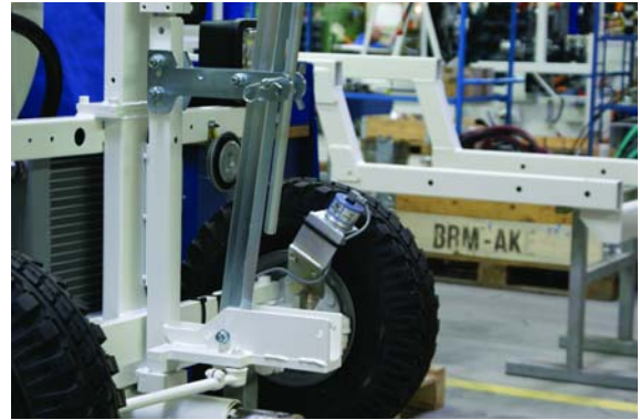
Fig 2: WDG 58 encoder employed on the front wheel
