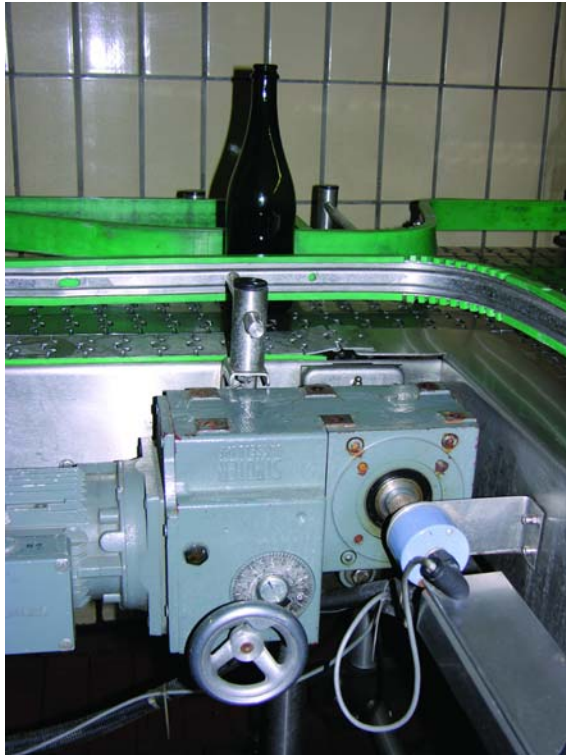
Fig 3: Measurement of the bottle position for optimal quality inspection
